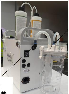
Facing the back of the Aquaglo device, connect Waste Outlet on the **right side**.
