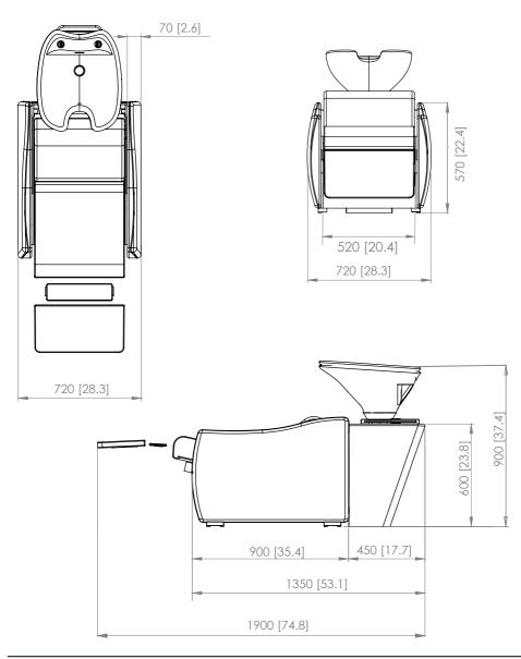
DIAGRAM A All measurements are in mm (inches).
